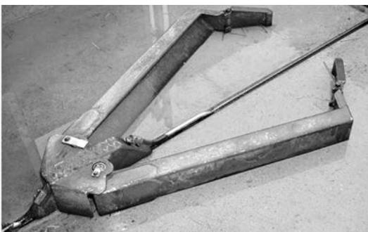
Abb. 1: Neu entwickelter falt-Kombi-Schieber Fig. 1: New design of V-shape scraper with folding ends
