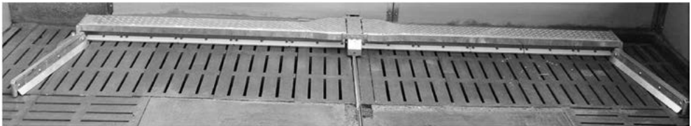
Abb. 2: Neu entwickelter Kombischieber Fig. 2: New design of tilting scraper with folding ends
